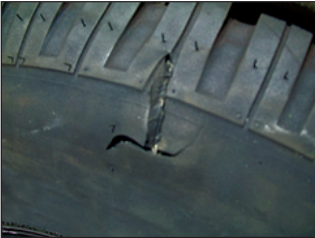
Condition – Sidewall cut
