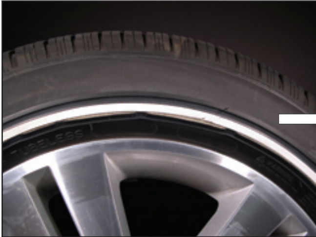
Condition – Sidewall coverstrip split Tire Condition Code – TA4
