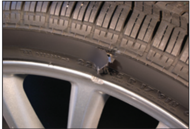
Condition – Sidewall snag Note: additional evidence of damage to the wheel
