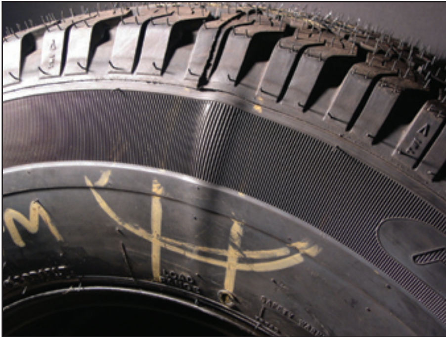
Condition – Sidewall bulge Tire Condition Code – TA3
