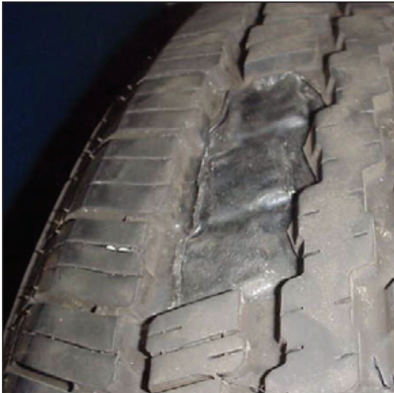
Condition – Tread chunk missing Tire Condition Code – TA5
