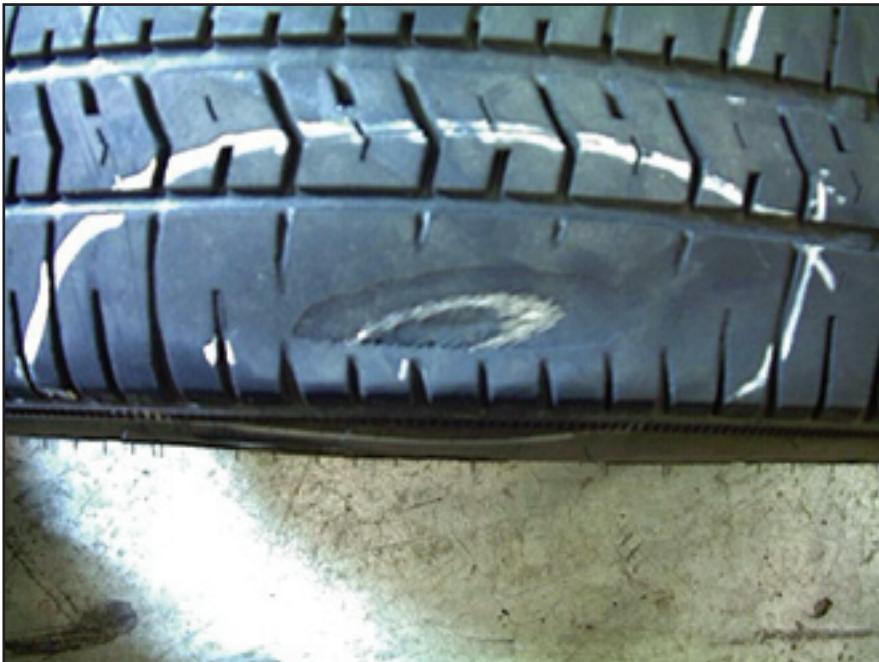
Condition – Separation in one spot on tread Tire Condition Code – TA1
