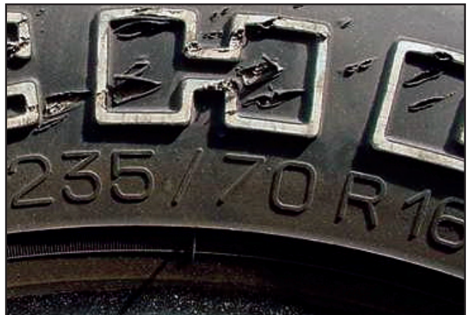
Condition – White sidewall veneer damage (example above shows damage from a pressure washer)
