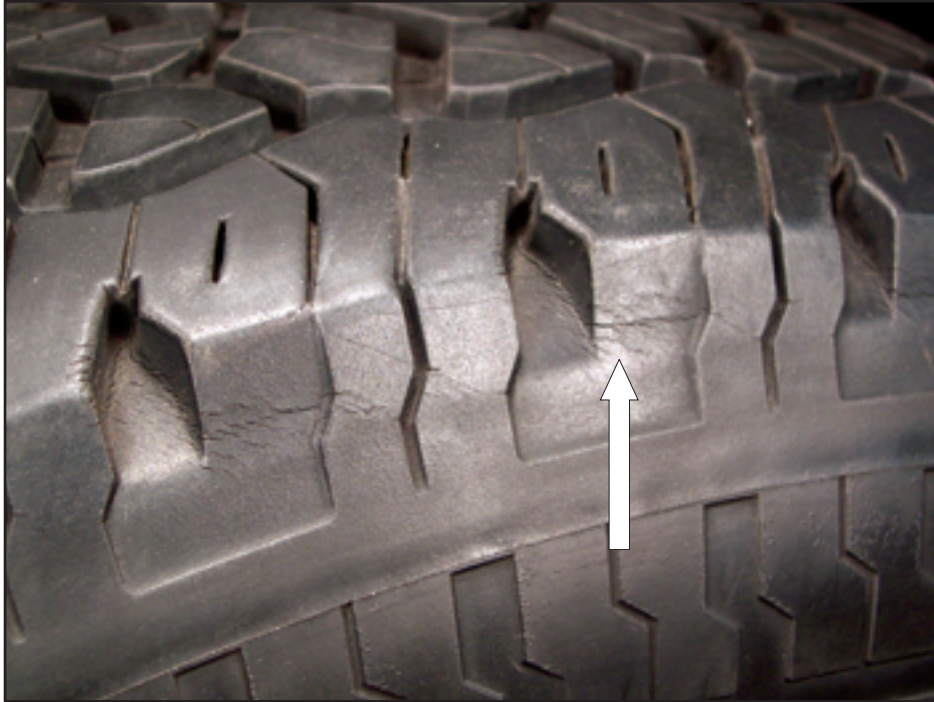
Condition – Cracks on shoulder Tire Condition Code – TA4
