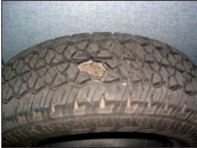
Condition – Tread chunk missing Tire Condition Code – TA5
