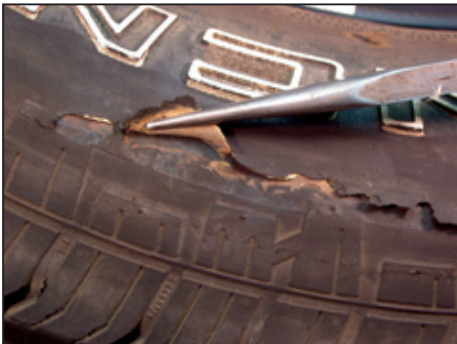
Condition – Sidewall delamination Tire Condition Code – TA4
