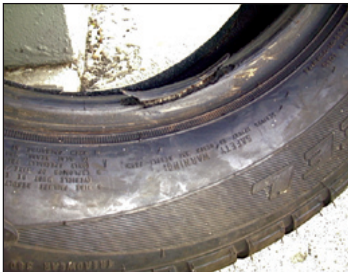
Condition – Torn bead, caused by improper mounting.
