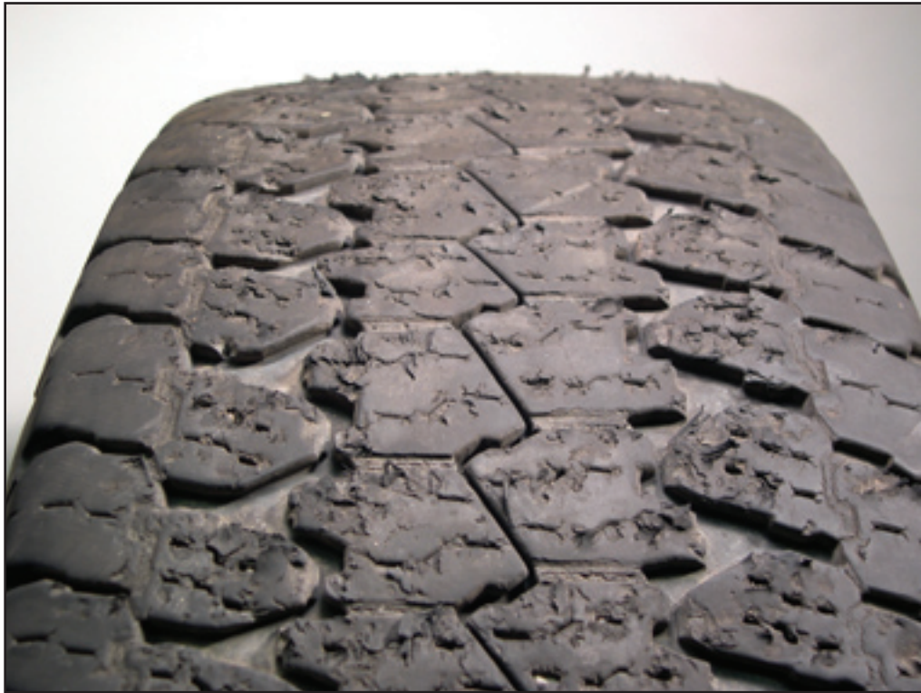
Condition – Tread damage as a result of rough service
