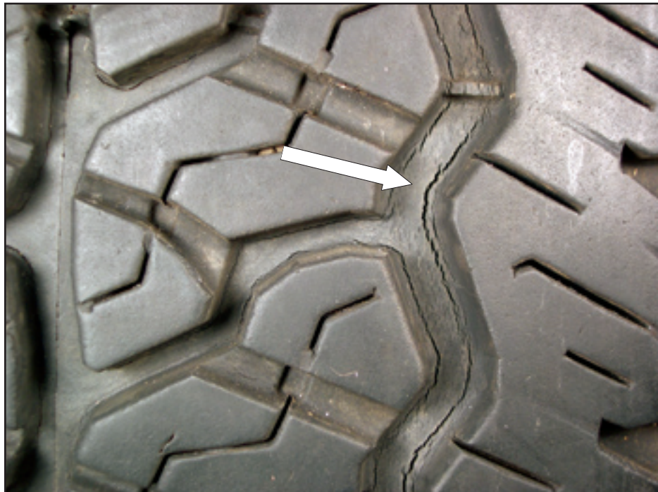
Condition – Tread cracking Tire Condition Code – TA4
