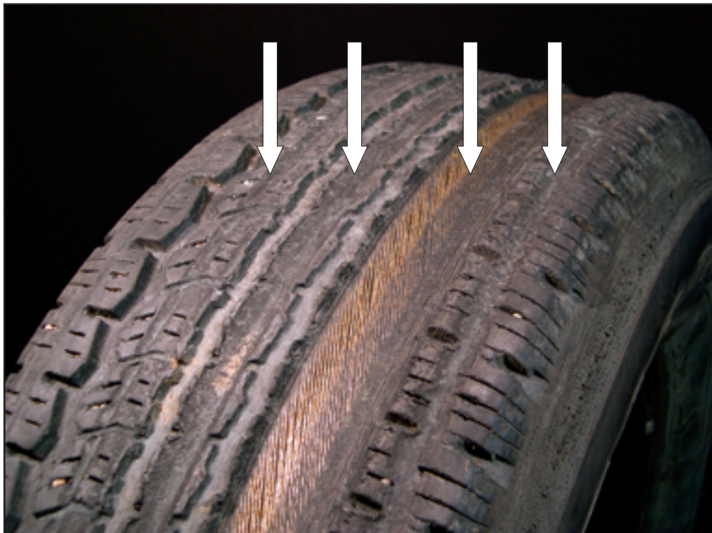
Condition – Tread damage from vehicle contact/rubbing against the tire. Note the deep grooves gouged into the tread area
