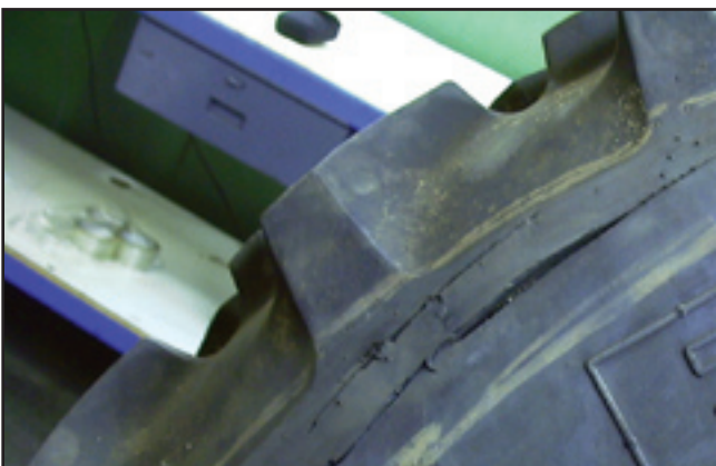
Condition – Obstruction cut in sidewall
