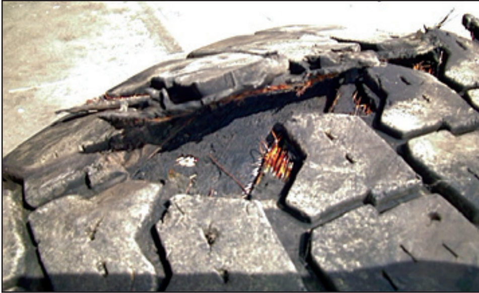
Condition – Crown area separation Tire Condition Code – TA1
