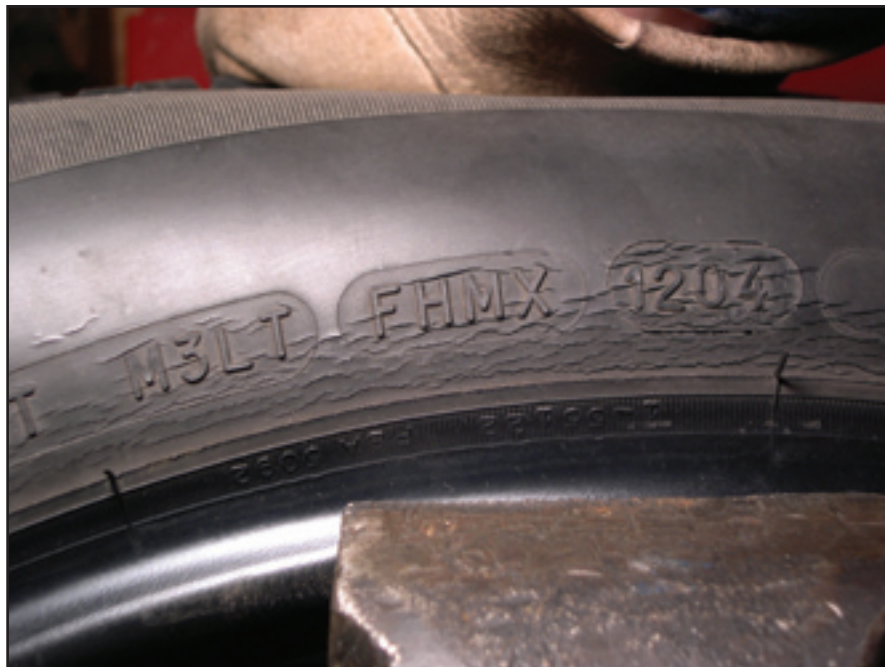
Condition – Sidewall cracking Tire Condition Code – TA4
