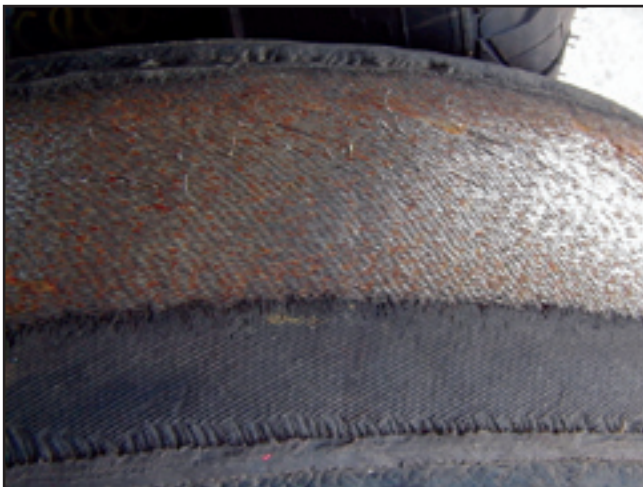
Condition – Tread delamination Tire Condition Code – TA1
