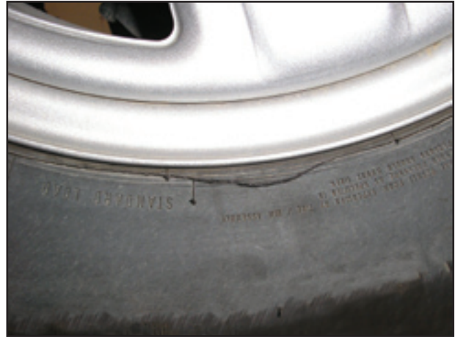
Condition – Sidewall cracking Tire Condition Code – TA4
