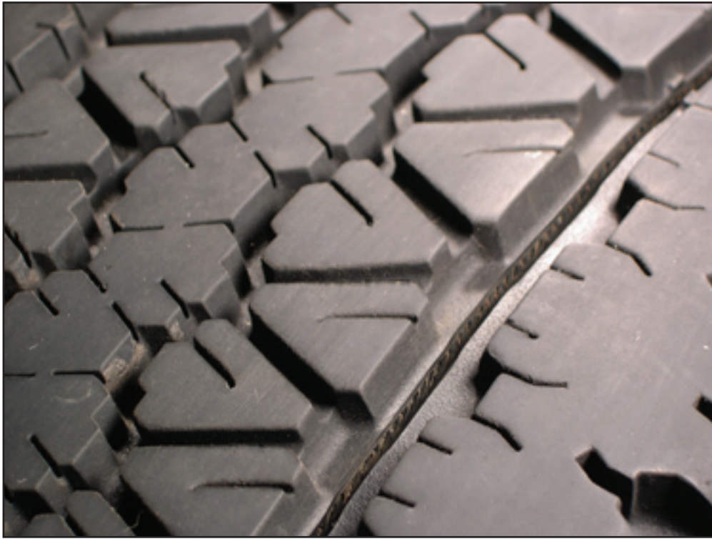
Condition – Cut in tread groove
