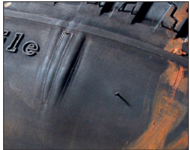
Condition – Open sidewall splice Tire Condition Code – TA4
