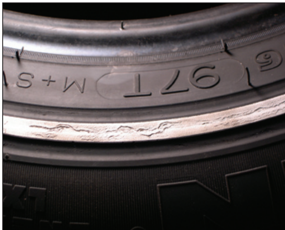
Condition – Premature sidewall deterioration Tire Condition Code – TC8
