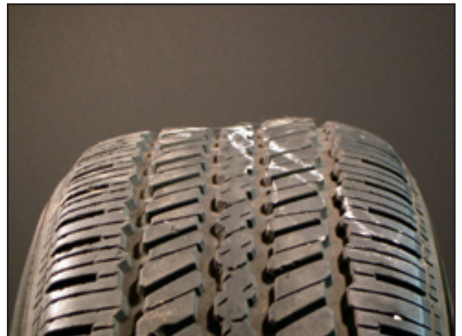
Condition – Distorted tread/tread separation Tire Condition Code – TA1
