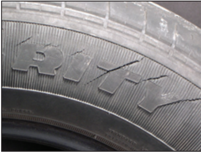
Condition – Diagonal sidewall cracking Tire Condition Code – TA4
