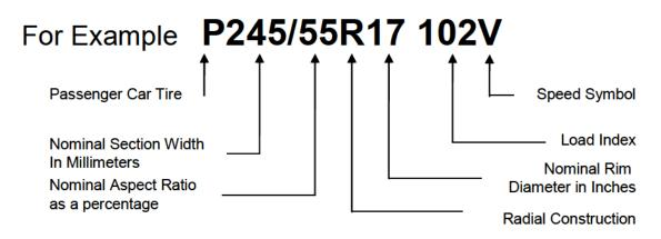
**Load Index Number,** a numeric code which indicates the maximum load carrying capacity of a tire at the maximum cold inflation pressure.
